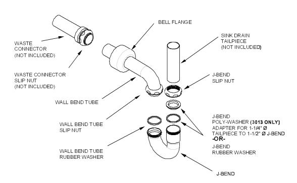
Hand tightening all the slide nuts should provide a good seal to joints
