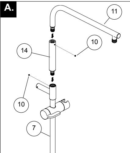
**A.** Assemble the height extension (14) to the shower column (7). Assemble the overhead shower arm (11) into the height extension. Tighten with set screws (10).
