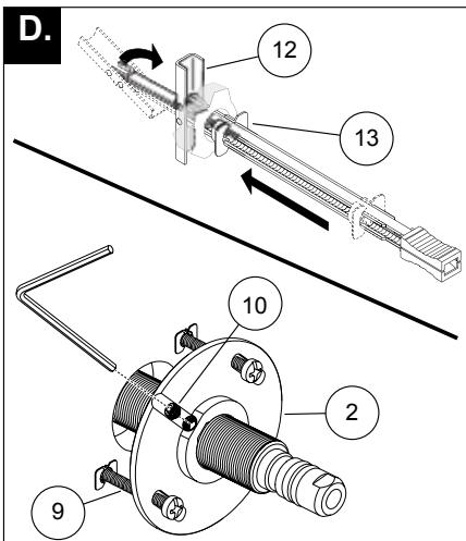
**D.** Install anchor assembly (12) by inserting metal channel through hole. Hold ends of straps and pull toward you until channel rests flush behind wall.
