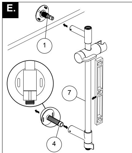
**E.** Insert the lower mounting post (4) into the lower post of the shower column (7).
