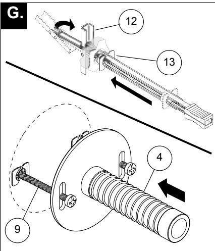
**G.** Install anchor assembly (12) by inserting metal channel through hole. Hold ends of straps and pull toward you until channel rests flush behind wall.
