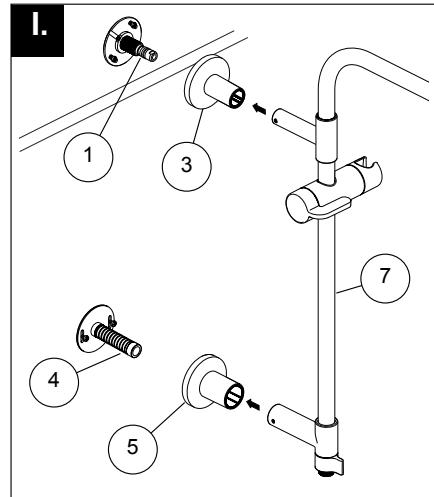
**I.** Assemble the upper escutcheon (3) and lower escutcheon (5) onto the upper and lower post of the shower column (7), respectively. To ease in installation, lubricate the escutcheon o-rings with water.
