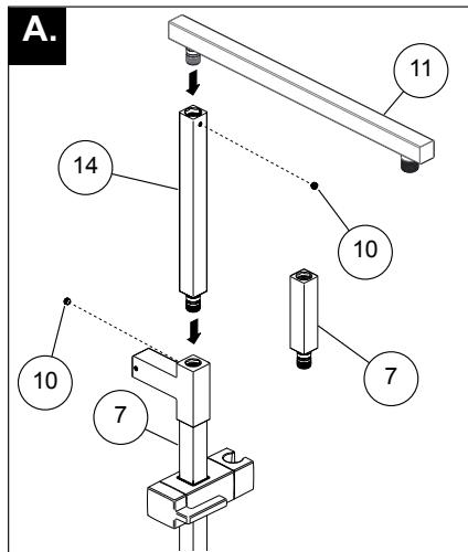
**A.** Remove existing height extension from shower column (7). Assemble longer height extension (14) to the shower column (7). Assemble the overhead shower arm (11) into the height extension. Tighten with set screws (10).
