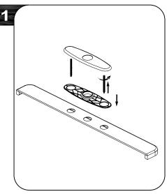
Screw bolts to the escutcheon. Insert escutcheon assembly through the base plate and the holes of the sink.
