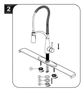
Insert faucet body through the hole in escutcheon. From underneath sink, hand tighten mounting nuts (1). Install washer (2) and (3) onto the threaded mounting shank. Thread nut (4) onto mounting shank. Do not overtighten.
