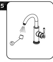
Important: after installation is completed, turn on hot and cold water supplies. Remove aerator ①. Turn faucet handle to the warm position where it mixes hot and cold water. Flush water lines for one minute. Check for leaks.Retighten any connections if necessary.Reinstall the aerator tightly.
