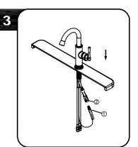
From underneath the sink, align block ① and tabs ② on quick connects. Push quick connect housing firmly upward and snap onto receiving block. Pull down moderately to ensure connection has been made. If it is necessary to remove quick connect, squeeze tabs on hose between index finger and thumb, then pull down to disconnect.
