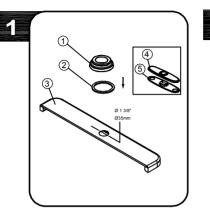
Shut off water supplies.Clean sink surface. Place washer 2 and flange 1 on the sink 3.If you do not use flange,please use escutcheon 4 and gasket 5 to replace flange and washer.
