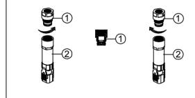
The faucet ships with a 1.5GPM aerator installed. An optional 2.2 GPM aerator is also included in the box. To switch the flow rate of the faucet: 1. Disassemble the quick connect assembly by
