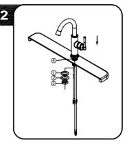
Place faucet through the hole in top of sink. From underside,assemble rubber washer ①,metal washer ② and nut ③ onto long shank ④ and tighten nut ③. Firmly tighten the nut ③ to metal washer ②. Do not overtighten.
