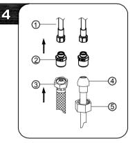
Make connections to water lines with 3/8" female compression supply hoses ①.
