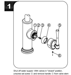
Shut off water suppi/ .With valves in "closed" position, unscrew set screw (6) and remove handle (5) from valve stem (2). Loosen the screw (3) from valve stem (2). Loosen the cap (4) from the cartridge nut (1).
