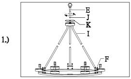
Step 1: Assemble the fixture by attaching arms (I) to the ring. At three points the arms can be locked down to screws and secured with knurled thumb screws (F) provided. As you tighten down the arm with electrical wire, note that wire must be pulled through the collector (K). Attach coupler (J) and stem (E) to secure the assembly.
