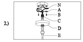
Step 2: Remove mounting bracket (A) from fixture and install to electrical box. Attach appropriate amount of chain to loop to achieve desired mounting height. Thread wire through every 3rd loop of chain. Remove ring from loop and slide down chain. Place canopy (D) onto chain and let slide to top of fixture. Wire fixture to wires in outlet box. Copper wire is for Ground. Pull canopy through screw ring up chain to ceiling and tighten securely.
