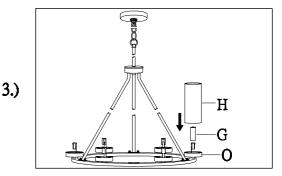
Step 3: Attach the candle cover (G) over the socket and press glass onto the cup (O) to secure.
