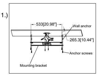
Step1.Remove mounting bracket from fixture and install to electrical box.Mark where the narrow end of the keyhole slots on the bracket meet the wall.Remove mounting bracket from wall.Drill holes using 1/4" ± drill bit where marked.Install mounting bracket to outlet box and hammer anchors into drill holes.Thread anchor screws into wall anchors until wall pate is flush with wall.
