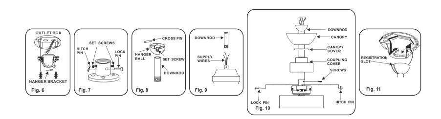
Follow the steps below to connect the fan to your house supply wires. Use the wire nuts supplied with your fan. Secure the wire nuts by wrapping the connection with electrical tape.
