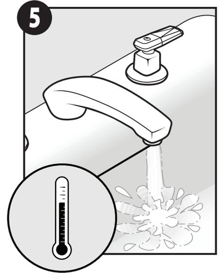
If temperature is over (>) 120°F (49°C) go to 6. If less (<) 120°F (49°C), installation is complete.
