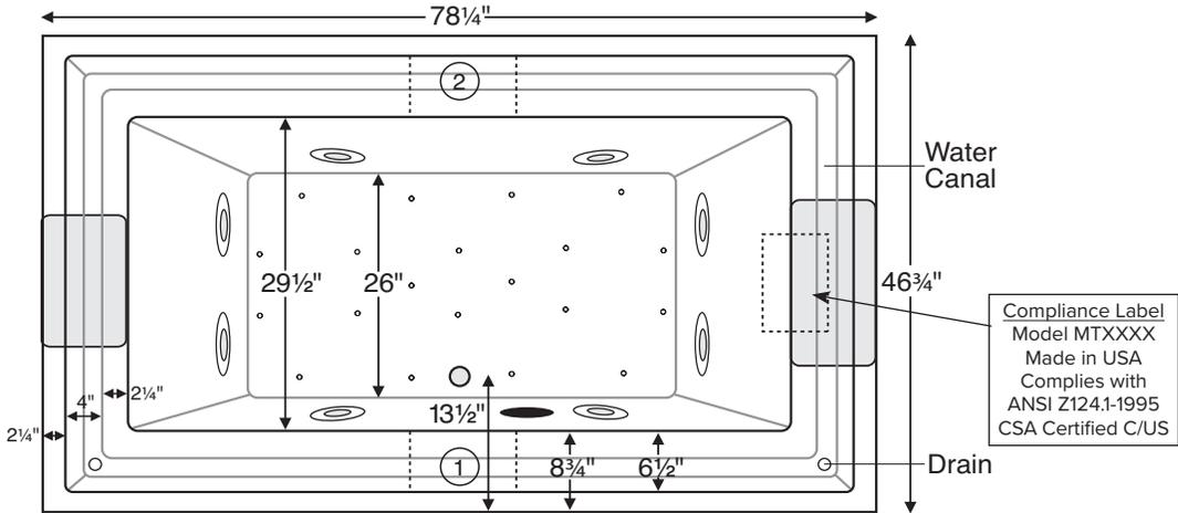
Dotted lines indicate a raised, level deck area which is optional for valves and required for whirlpool. Air bath control must be mounted adjacent to the tub and is shipped loose when ordered without deck plugs. Shown with Air Massage and Ultra Whirlpool Package.
