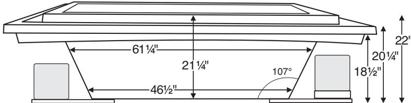
**IMPORTANT:** Air baths and tubs with a pre-leveled foam base or frame system add 2-3" to overall tub height.
